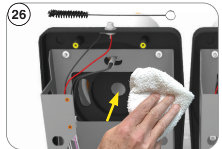
26. Spray warm water into Cooling Drum openings to help loosen debris. Then clean inside and around using a brush and towel.
