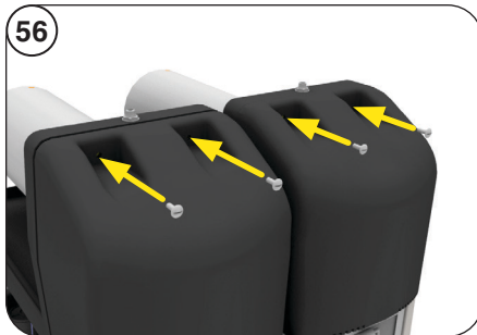
56. Replace Auger Motor Covers using 2 screws in each.
